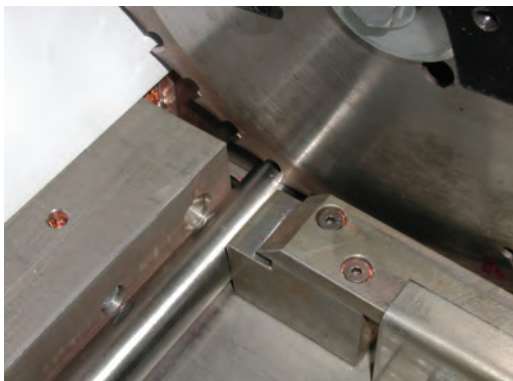
1. Saw off the tubes rectangularly.
