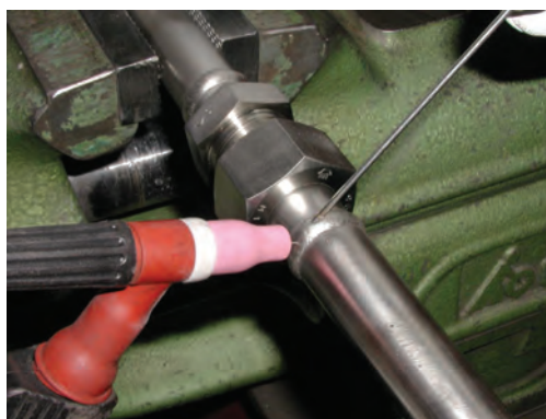
4. Unscrew the clamping nut and weld the tube connections. Pay attention to the negative pole.
