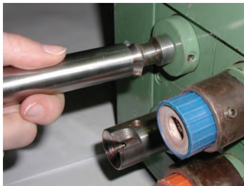
2. Deburring of the bores Chamfer the tube edges according to DIN EN ISO 9692-1.
